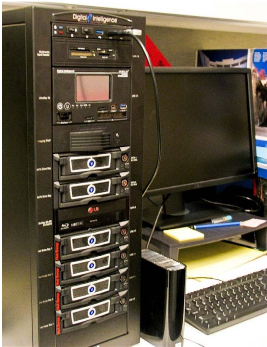
Figure 5. Digital forensic equipment used to analyze the content of electronic records at the Getty Research Institute. Photo provided by the Getty Research Institute.
